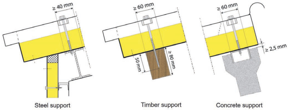
Figure 24: End support conditions
