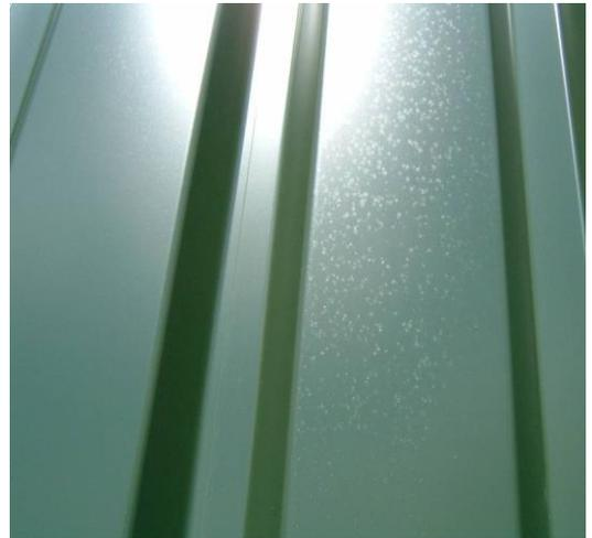
Visible effect: thin, white deposit (fig. D1 and D2)
