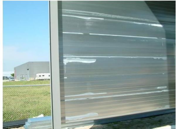
Visible effect: thin, white, powdery deposit (fig. A1 and A2)
